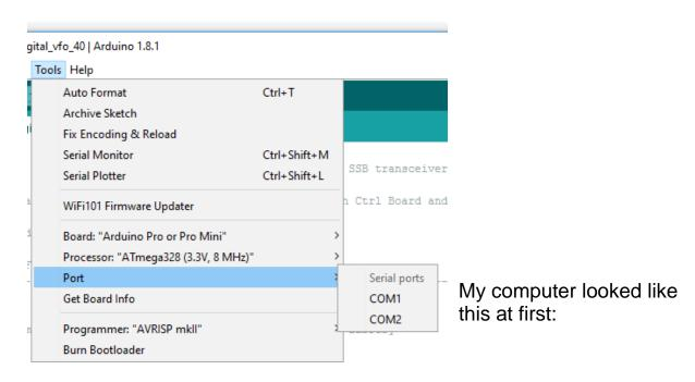
Now insert the FT232 adapter into a spare USB port on your computer. A new port should appear on the software.
