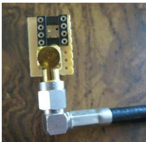
Mount the SMA Cable and connect the other end to the Adaptor.
