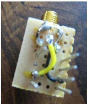
On the under-side, as shown, clip pin 7 of the IC Socket.
