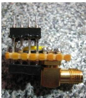
I soldered a machined socket to the wire wrap pins so that it would insert into my PC board more easily.
