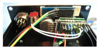
Note: If no header pin was placed on the Sandwich, you may clip off the 2 pin connector and solder the wires on the Sandwich I2C buss.
